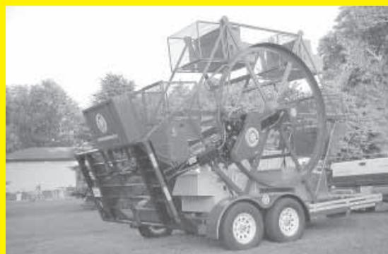
**Unit hydraulically folds down for transport. No tools are required for either setup or take down.**
