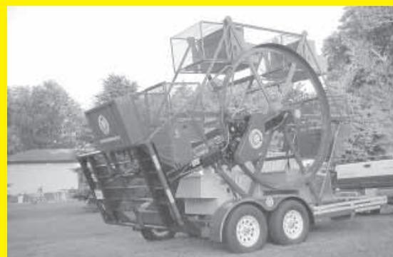
**Unit hydraulically folds down for transport. No tools are required for either setup or take down.**
