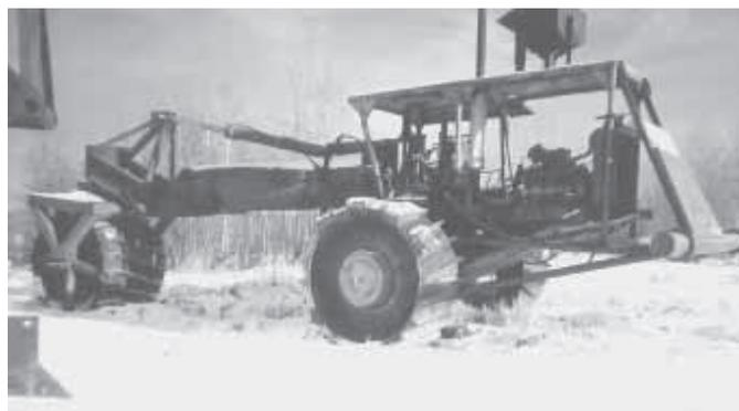
**“Tree-Crusher” rolls over and kills trees with 4-ft. wide, lugged drive wheels. Grass seed is spread in front of the wheels so they’re pushed down to planting depth by the wheels.**
