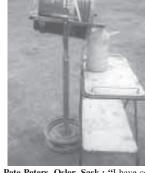
Pete Peters, Osler, Sask.: "I have come up with a stand that makes it easy to pour oil or other substances easily. It consists of an old wheel rim with a piece of steel pipe welded onto it. The strap iron bracket on top is made to hold a 5-gal. bucket. You can control the pouring with one hand, which leaves the other hand free to steady the container you're pouring into."
