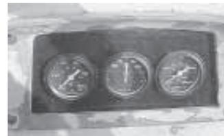
black and attached an old set of automobile gauges for amps, temperature and oil. It was pretty easy and they work just as well as the originals."
