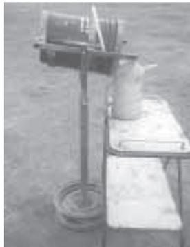
**Pete Peters, Osler, Sask.:** "I have come up with a stand that makes it easy to pour oil or other substances easily. It consists of an old wheel rim with a piece of steel pipe welded onto it. The strap iron bracket on top is made to hold a 5-gal. bucket. You can control the pouring with one hand, which leaves the other hand free to steady the container you're pouring into."
