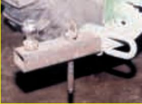
This 8-in. length of rectangular tubing has a bolt-on ball hitch at one end. By pinning the tubing onto my tractor drawbar I can quickly switch to a ball hitch without any tools. **(Eric Webster, 697 Warburton Rd., Lansdowne, Ontario, Canada K0E 1L0 ph 613 659-2450)**
