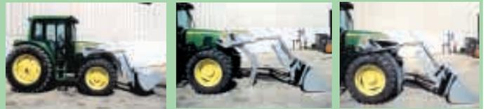
To dismount loader, you flip up a steel plate that fits inside a bracket on front of tractor. As you back up, "tower stabilizer" automatically drops to hold loader upright on ground.
