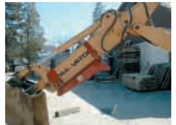
Extendable "thumb" turns backhoe into a true mechanical hand, says manufacturer.
