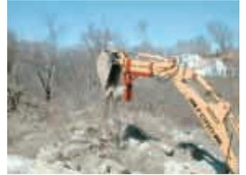
Thumb makes backhoe ideal for moving scrap metal or logs. Both the thumb itself and the arm it's attached to offer multiple positions for different needs.
