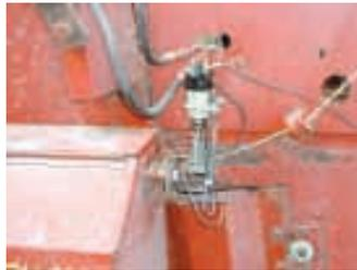
**Device bolts onto baler between twine box and twine applicator tubes and is connected to a remote switch in the cab.** started selling a few of my twine brakes to local farmers. I offered to take the product back if there were any problems, but I haven't got one back yet."
