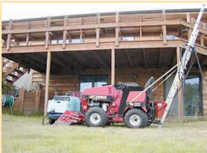
To attach ladder, Bergman ran a steel rod through bottom rung and then through the lift arms on tractor 3-pt. Then he ran two support straps up to a rung about halfway up ladder.
