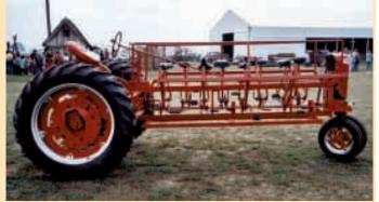
Rubison removed the engine and mounted two banks of four bicycles back to back. He says just one person pedaling can move the tractor.
