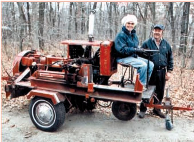
Gerald Krob converted his wood splitter to this self-propelled model that's also equipped with a 32-in. buzz saw.
