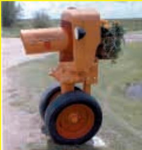
I unbolted the front end of the tractor and bolted on a fake radiator that I made from steel plating. The mailbox itself is a short length of 10-in. dia. auger tube. After making a door for the mailbox, I welded a bracket on back of the grill to hold a flower basket. The tractor mounts on a length of 3 1/2-in. sq. tubing anchored in cement 5 ft. underground. (Allen and Cindy Clow, 3739 230<sup>th</sup> Ave., Lancaster, Minn. 56735)
