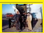
My son Todd and I mounted an 8-ft. frontmount snowblower in place of the header on a stripped-down 1972 Gleaner K combine, which we bought for \$560. We removed the grain-cleaning components and mounted a right angle gearbox in place of the threshing cylinder. Then we installed a Cat. II quick hitch on the feederhouse. The chain-driven snowblower is controlled by the clutch that originally operated the header.
