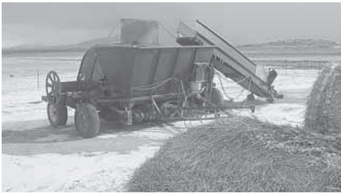
**Kent Durfee modified an old Eberhardt Silopresse bagger. His silage trucks dump onto a conveyor belt that feeds haylage into hopper.**
