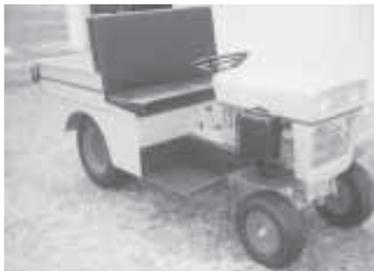
**George Hone's 2-seater "get around" was built from an old Bolens lawn tractor. It's complete with a cargo box on back.**
