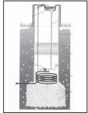
**Freeze-proof waterer uses a 12-in. PVC well casing, with the lower end set below the frost line. Coiled water supply hose allows entire drinker assembly to be removed from PVC pipe without unhooking hose.**
