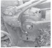
Hatton plugged side vent hole (1) and put vent on top (2). Pipe now feeds oil to gearbox (3).
