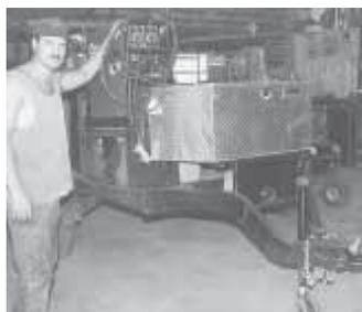
**Lloyd Meffert built this 2-wheeled “repair trailer” out of an old camping trailer:** an air compressor, a handyman jack, a set of mechanic's tools, different kinds of welding rods, chains, binders, come-alongs and a sledge hammer.
