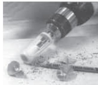
**Pro-Sharp can be slipped into a drill chuck to sharpen a pencil in just seconds.**
