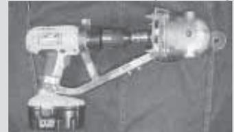
with this 'wire twister' that's powered by a standard DeWalt 18-volt cordless drill. It grabs one end of the wire and twists it around itself a few times. You manually put all the wires around the post and then give them a half turn. Then you use my invention to fin-
