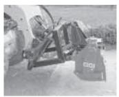
Universal mounting plate for skid loaders is equipped with a hydraulic-driven pto that lets you use any pto-driven, Cat. I tractor attachment on a skid loader.
