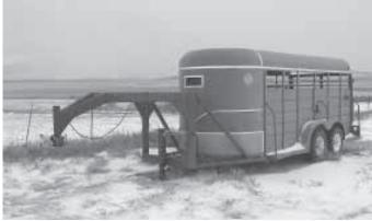
Kent Durfee can pull his stock trailer with either a bumper hitch or a gooseneck hitch, thanks to the adapter he made for the trailer.
