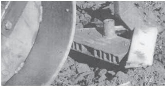
Design of the opener and firming roller assures that all seed is placed at precisely the same depth, says inventor LeRoy Richard.
