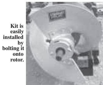
**Kit is easily installed by bolting it onto rotor.**
