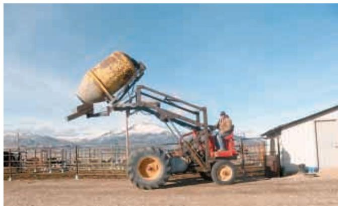
"With tank mounted on lift, we can raise it up to 9 1/2 ft. high to dump," says Kent Durfee.
