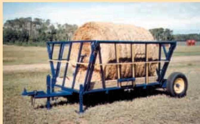
Pins are inserted into either end of bale, then winch is used to pull bale into the feeder.
