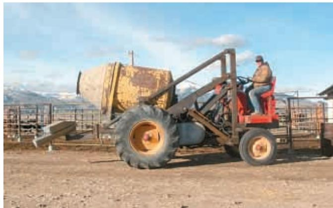
Weight of mixing tank is centered over drive wheels, which aids in steering and also makes rig more stable.
