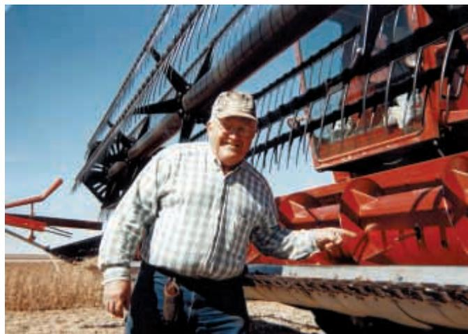
In addition to a more even crop flow, added fingers also let Roetman raise the reel up to reduce shatter loss, letting augers and fingers pull the crop in.
