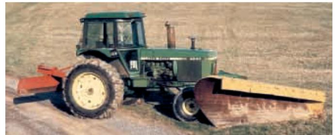
In addition to front blade, Allison's 4240 also has a back blade that's used to pull snow away from buildings.
