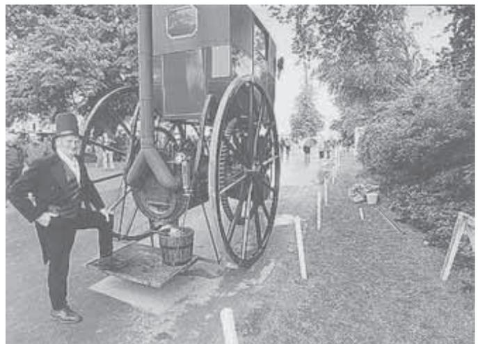
The 8-ft. dia. wheels on Trevithick's 1803 steam-powered vehicle were designed to smooth out bumps on the road to avoid shaking, which might put out the fire.
