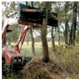
Tree is rocked back and forth to loosen the roots before it is pulled out.
