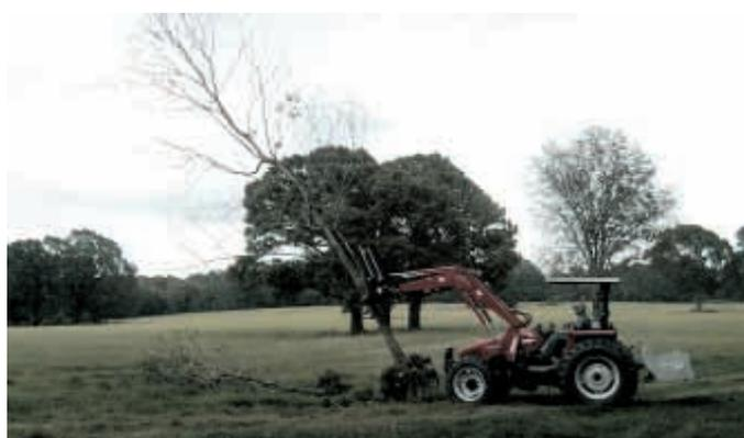
Lang's puller removes trees without leaving holes like a dozer or stumps like a tree cutter.
