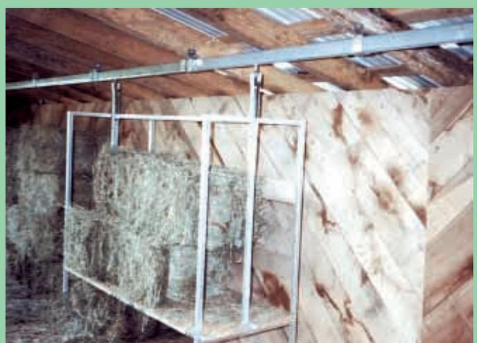
Overhead track allows bales to be moved easily from one end of barn to the other. One shove is all it takes to move carrier the length of barn.
