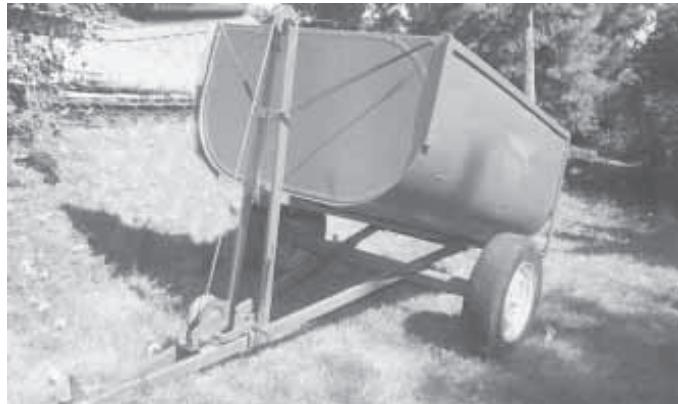
Two-wheeled, pull-type dump trailer was built out of a 265-gal. fuel oil tank and a boat winch that mounts on the tongue. To dump the load, Prom simply cranks the winch.
