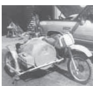
To make the motorcycle sidecar, Wiederrick used the rear wheel from a motorbike and the front rack from a 4-wheeler. Sidecar has a padded seat and arm rests.
