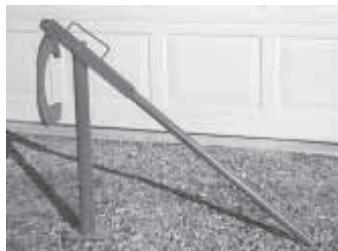
Manual post puller is designed with a "C"-shaped steel hook that hinges at end of a 34-in. long metal handle. As you pump the handle, the hook "bites" into post.
