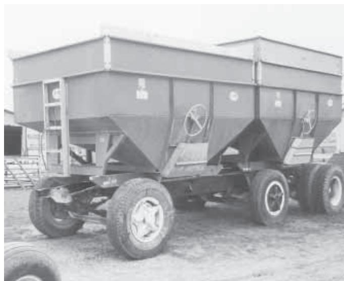
Walter Baldner mounted these 525 and 250-bu. gravity wagons on the frame of an old tandem axle truck. "By pulling a 350-bu. wagon behind the two boxes, I can haul about 1,100 bu. at a time," says Baldner.
