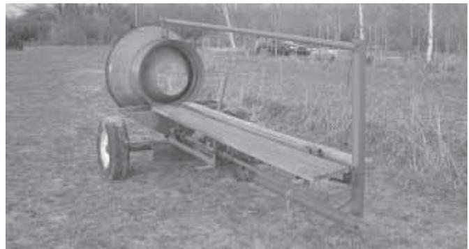
As tree leaves cone, it drops onto a wooden platform that extends the length of the machine.
