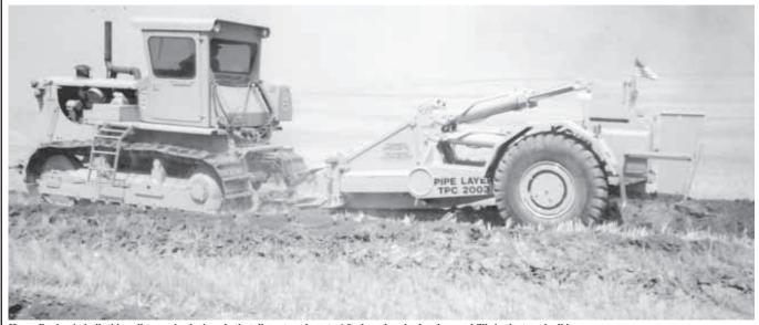
Harry Benjamin built this pull-type pipe laying rig that digs a trench up to 6 ft. deep, lays in the pipe, and fills in the trench all in one pass.
