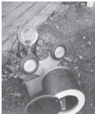
Belt-driven by an electric motor, drum rotates to mix soil.
