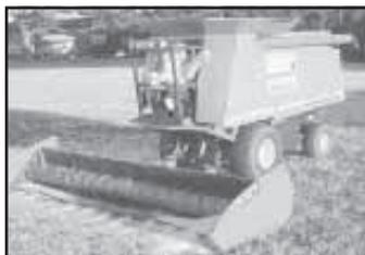
Mini combine's header and unloading auger work like the real thing.
