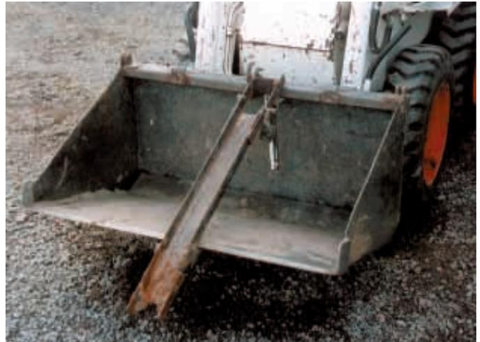
A length of 4-in. wide channel iron on bucket is pointed inward at one end. It bites into roots so that Johnson can raise the bucket and lift trees and brush out.
