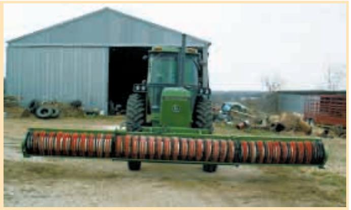
Machine is equipped with a 20-ft. wide stripper head on front with a 3-pt. mounted grain tank on back.
