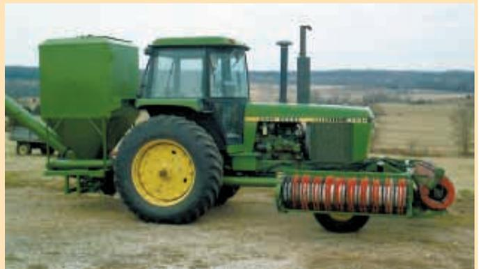
Platform that stripper head mounts on folds to a transport width of 12 ft.
