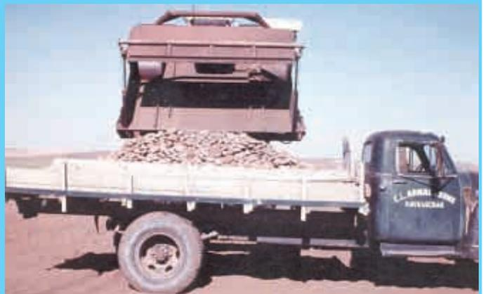
Two 4-ft. hydraulic cylinders raise box high enough to dump into truck. A second set of smaller cylinders tips hopper to dump it.
