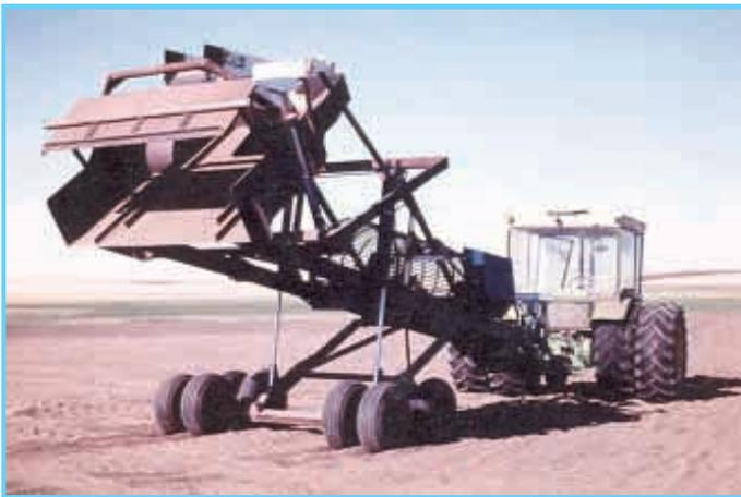
Clifford and Clarence Arnal enlarged the hopper on their Harley rock picker and designed a new scissors-type lift to dump hopper into truck.
