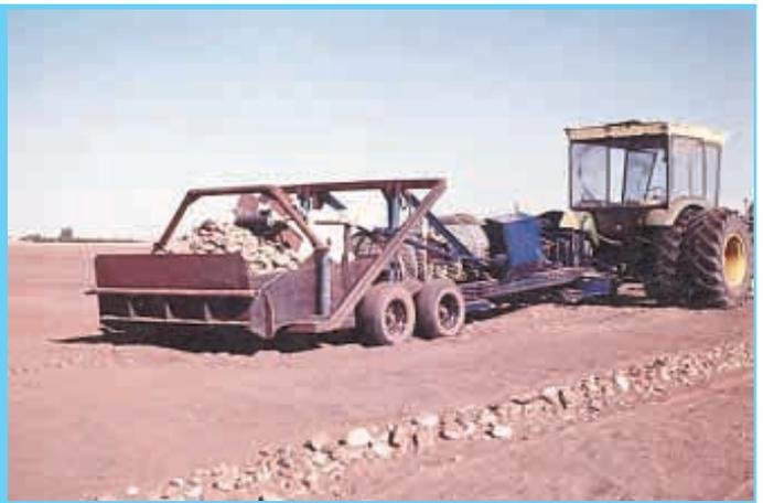
Before using the rock picker, they windrow rocks with either a tooth rake or a roller rake. Modified picker handles stones up to about 14 in. diameter.
