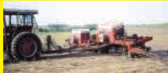
After we attached the two planters together, we had to devise a hitch that would pull both of them. An offset hitch allowed us to save more money by using only one marker, but the other planter needed 500 lbs. added to balance out the weight. So far our IHC 1466 has had no problem pulling it and we are very pleased with the results. **(Wayne Wesley & Tim Wesley Dressen, Dressen Farms, 1597 Co. Rd. P25, Kennard, Neb. 68034 ph 402 427-7183)**
