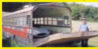
is raised and lowered with an electric winch that runs off the bus's 12-volt electrical system.
