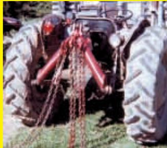
sists of a pair of 4-in. dia., thick-walled pipes welded together and reinforced at the top. A horizontal pin is welded onto the bottom of each pipe and on top there's a bracket that hooks up to the tractor's 3-pt. top link. I welded on four hooks where the pipes come together and hook chains onto them.
