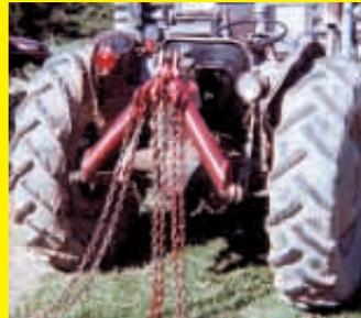
sists of a pair of 4-in. dia., thick-walled pipes welded together and reinforced at the top. A horizontal pin is welded onto the bottom of each pipe and on top there's a bracket that hooks up to the tractor's 3-pt. top link. I welded on four hooks where the pipes come together and hook chains onto them.
