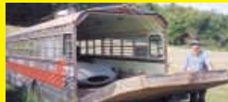
is raised and lowered with an electric winch that runs off the bus's 12-volt electrical system.
