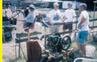
jack cylinder and fits into a wooden plate inside the horse. The whole effect is like that of a horse going up and down on a merry-go-round. **(Lloyd Mardikian, 25012 Trails End Road, Spooner, Wis. 54801 ph 715 468-2384)**
