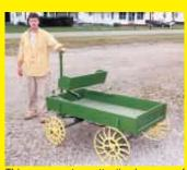
This wagon got my attention because of the unique wheels. Designed to look like an old horse-drawn wagon, the wheels are made from rotary hoe wheels with a band of steel around the outer teeth. (C.F. Marley, Nokomis, III.)
