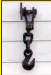
out of pieces of strap iron and attached it to a 1/2-in. chain link with a hook from a broken load binder. You can attach the pin without a wrench but the chain can't come loose as often happens with a log chain. Very handy. (Ross Cochran, Lucas, Iowa)
