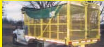
The twist on this product is that the cage is collapsible to allow access to the rear half of the bed, while still allowing the cage to be used. Within the rear half of the truck bed is a receiver that can be used to attach a gooseneck or kingpin hitch.
