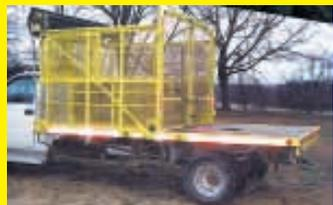
The truck bed is made of steel but could also be built of aluminum, as the customer desires. Additional modifications available include a hoist mounted under
