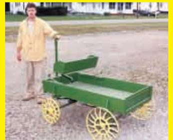
This wagon got my attention because of the unique wheels. Designed to look like an old horse-drawn wagon, the wheels are made from rotary hoe wheels with a band of steel around the outer teeth. (C.F. Marley, Nokomis, Ill.)
