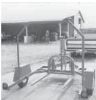
Single-bale trailer makes use of a used 3-pt. bale fork. A winch cable runs through a couple of pulleys and hooks to the lift for the fork.
