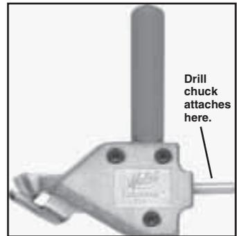
**TurboShear attaches to standard 3/8-in. or larger drill chucks. Once mounted on drill, it'll cut through galvanized sheet metal up to 20 ga.**
