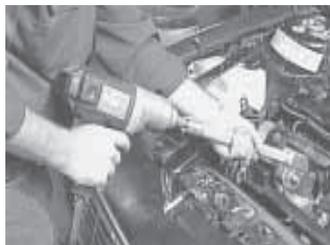
**Electric drill drives socket at end of handle, allowing wrench to apply tremendous torque to hard-to-reach bolts.**
