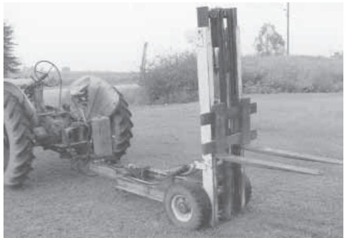
Marty Gallaher converted an old forklift mast into this 2-wheeled, pull-type rig. He can reach the forklift’s original hydraulic control levers from the tractor seat.
