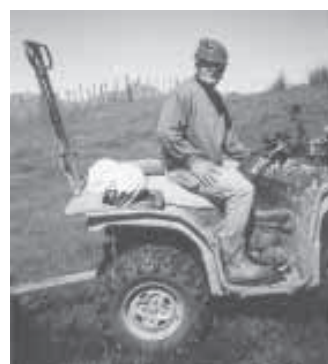
Safety helmet keeps ATV from starting unless driver is wearing helmet.
