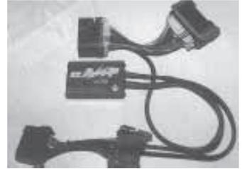
Plug-in chip reprograms engine's computer to alter time and duration of fuel injection according to load.
