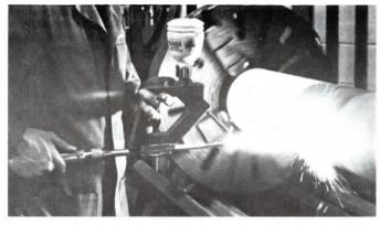
RotoTec kit includes gun and four modules of powder, including Xuperbond, the key to the process. It produces strong bond on all metals except copper and is the only powder needed for most jobs.
