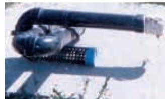
Oval-shaped water float is made up of four elbows and a couple pieces of 2-ft. long PVC pipe. Float holds intake nozzle about 4 in. from top of water and is perforated to keep screen from plugging up.
