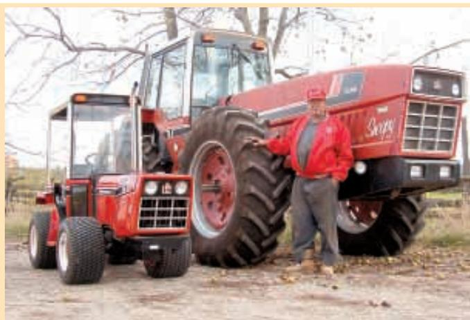
Carl Ruby modeled his homemade mini tractor after an IH 2 + 2 tractor. It's built roughly to 1/4 scale and powered by an 11 hp Yanmar diesel engine.
