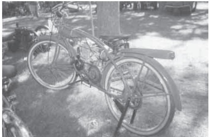
**Jim Parenteau converts older bikes to gas engine power, adding kick-start engines and handlebar-mounted, twist-grip throttles just like on real motorcycles.**
