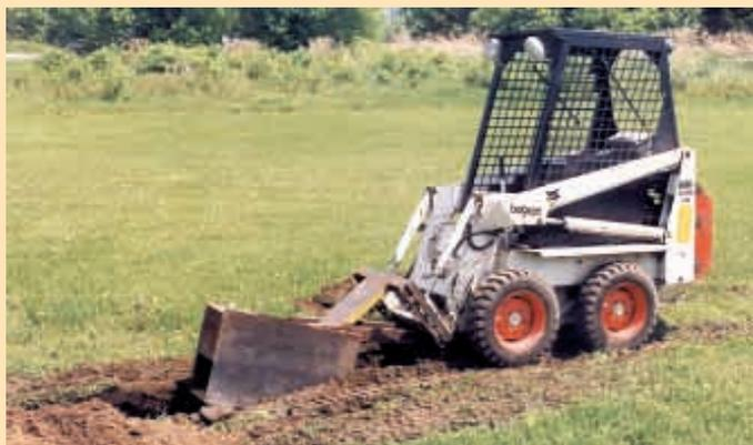
Johnson's 4-ft. long bucket digs a trench 10 in. wide and 14 in. deep. Back side of basket is partially open to allow trenching in either direction.
