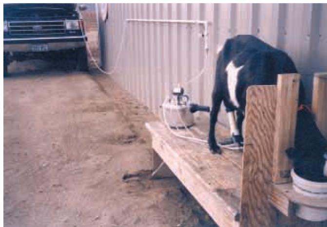
Engine vacuum provides the suction for Hoard's homemade milker.
