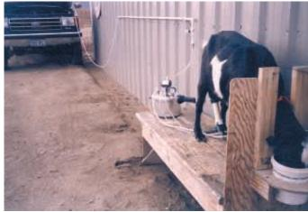
Engine vacuum provides the suction for Hoard's homemade milker.
