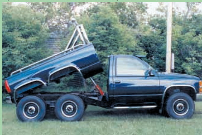
A 30-in. hoist powered off pickup battery allows truck to dump its contents.
