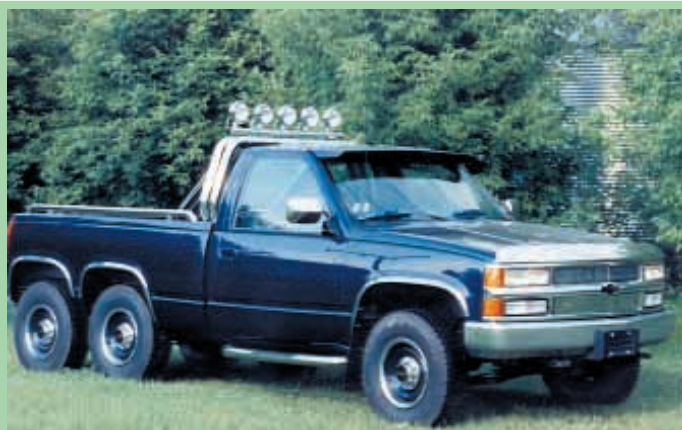
Heartt didn't need to lengthen the frame of his Chevy pickup to add a third axle, but he did add a second transfer case and the back half of another pickup box.
