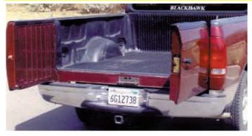
Two-piece "double door" tailgate opens from both sides, making it easy to load items onto bed.
